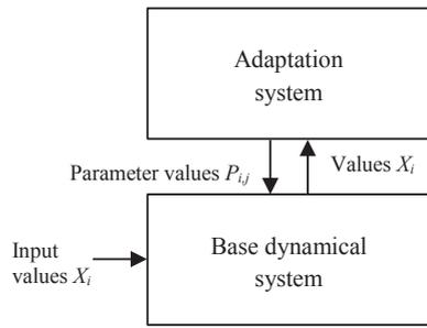
Fig. 3. Architecture of an adaptive dynamical system.
