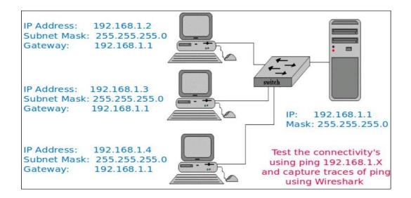
Connect four machines using Straight-Through cable to switch and router and then configure all using ip address, subnet mask and gateway address as shown in figure. Ping all the machines and capture ICMP packets in Wireshark tool.
