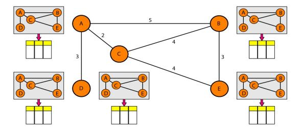
The figure shows a simple domain with five nodes. Each node uses the same topology to create a routing table, but the routing table for each node is unique because the calculations are based on different interpretations of the topology. This is analogous to a city map. While each person may have the same map, each needs to take a different route to reach her specific destination.
