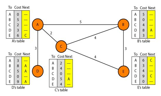
The table for node A shows how we can reach any node from this node. For example, our least cost to reach node E is 6. The route passes through C.
