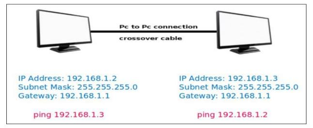
Connect two machines using crossover cable and configure it using ip address, subnet mask and gateway address as shown in figure. Ping from both the machines and capture ICMP packets in Wireshark tool.
