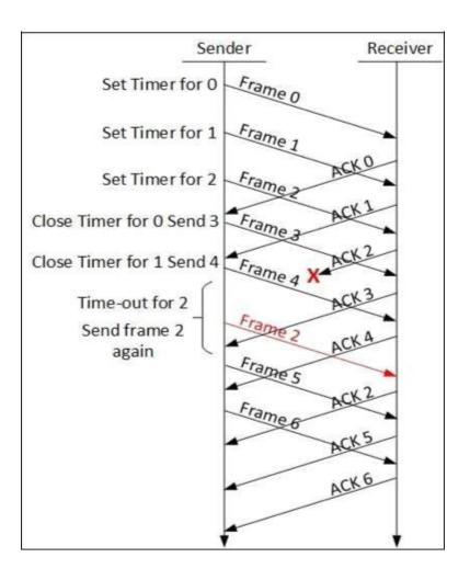
In Selective-Repeat ARQ, the receiver while keeping track of sequence numbers, buffers the frames in memory and sends NACK for only frame which is missing or damaged.
