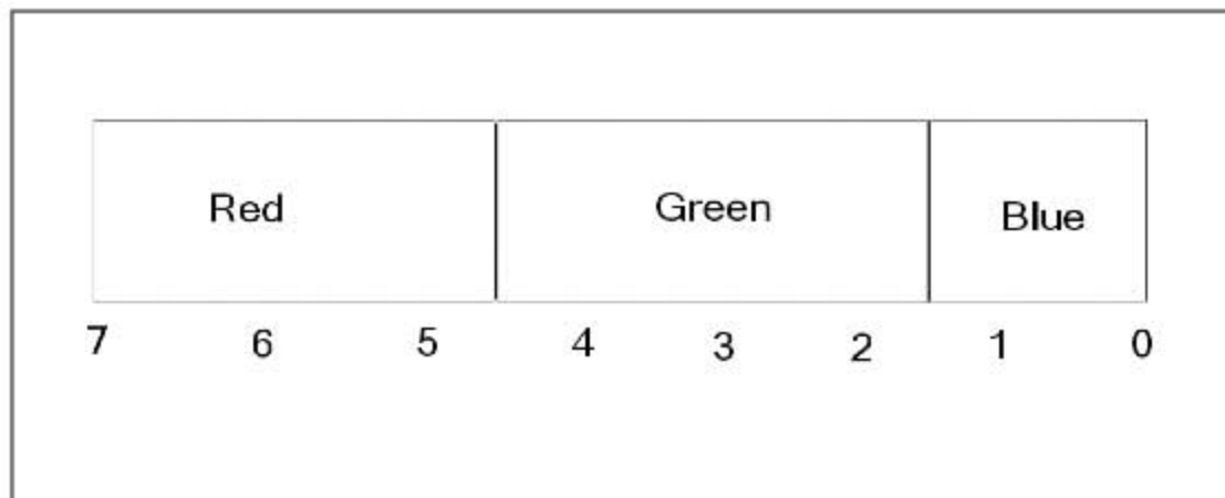
Figure 7.3 GL_UNSIGNED_BYTE_3_3_2 type with bit numbers for each component.
