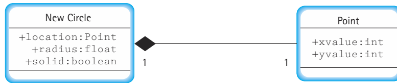
Figure 2.9 UML diagram showing has a relationship
