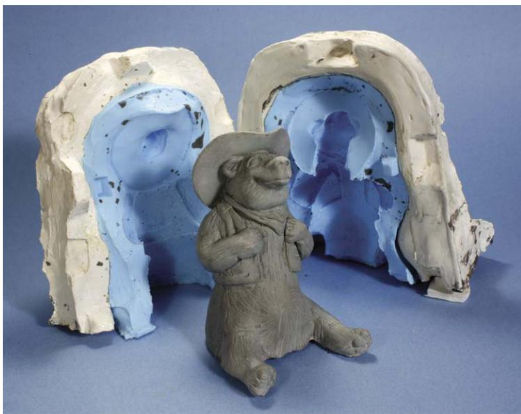
**Figure 9.10** Silicone rubber is the mold material of choice for professional makeup and stop motion artists.
