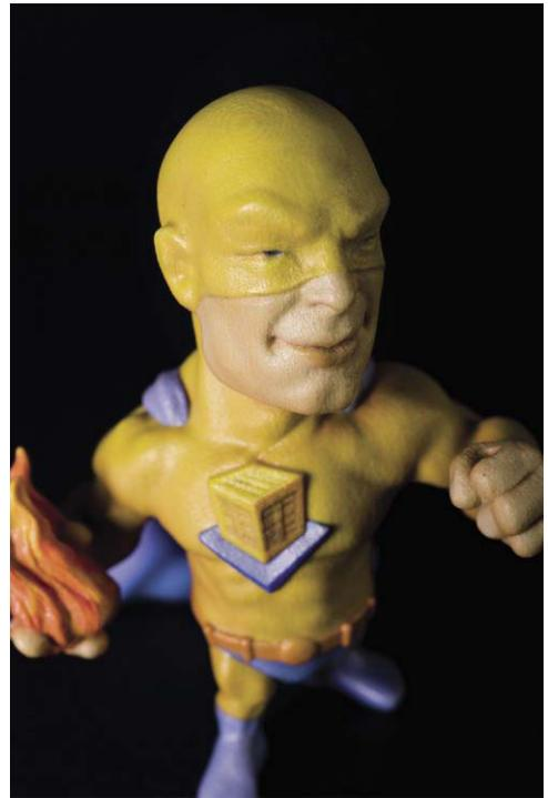
**Figure 11.14** *The Offload Man figure from the Offload studios 3D printer. Note the high degree of detail and subtle color that can be printed. Artists can use this system to create collectable figurines of their characters. A clay sculpture can also be scanned into the system in full color to create printer data for reproduction. Courtesy of [offloadstudios.com](http://offloadstudios.com). Photo by Laura Henderson.*
