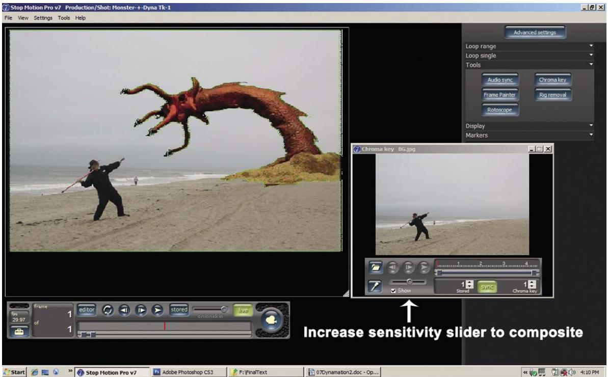
**Figure 7.19** Slide the Chroma Key slider to the point that the green disappears and is replaced by the background. Make sure the Show box is checked. Readjust the camera until the composition is just right. Clicking the Show box will toggle the composite on and off.
