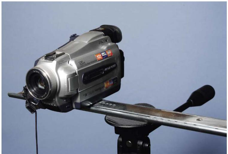
**Figure 10.21** Camera mounted to a drawer slider to create a smooth dolly move.
