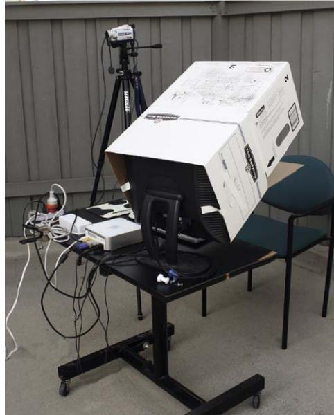
**Figure 2.5** If shooting outside, get a long extension cord for both camera and computer and make a sunshade for the monitor from a cardboard box. Mount your equipment on a roll-around table so you can easily move your setup.
