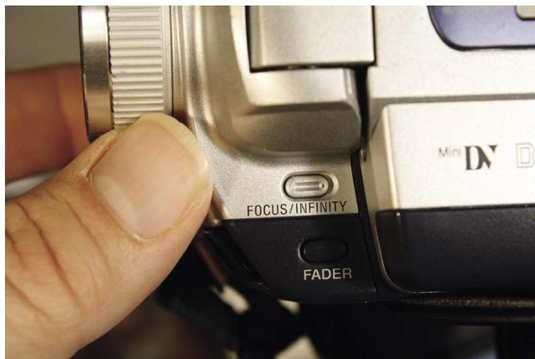
**Figure 2.6** Set your focus to manual, find a good focus, and leave it alone. This prevents auto focus fluctuations.
