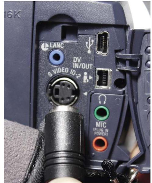
**Figure 10.9** Inserting the S video output of your camera into the black S video plug of the SMP Video Adapter will give you a slightly better video image.
