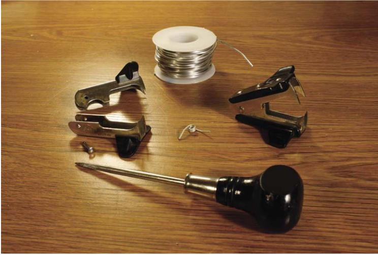
**Figure 3.2** Replacing the taut spring of this staple remover with soft aluminium wire allows it to be animated. The wire would be attached to the remover using super glue or epoxy putty.
