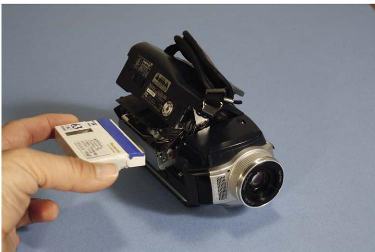
**Figure 2.2** Remove the tape from the camera.
