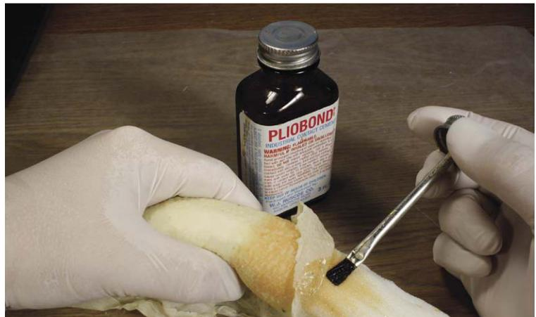
**Figure 7.10** Use Pliobond adhesive (available at local hardware stores) to glue the foam rubber together and attach the latex skin. Be sure to wear gloves.
