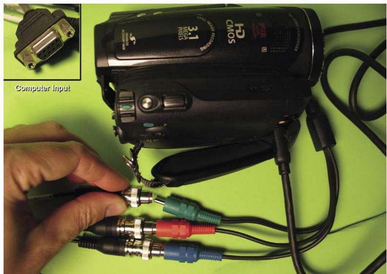
**Figure 10.10** A high-def camera connecting its red, green, and blue outputs to the computer via a Black Magic Design box.
