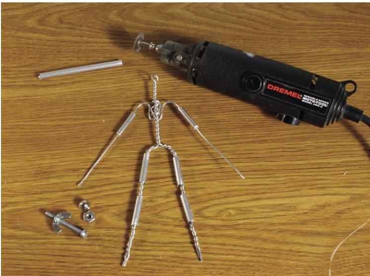
**Figure 6.11** The aluminum tubing can easily be cut with a motorized Dremel tool (be sure to wear eye protection). The braided wire and cap nuts for the feet can be attached with epoxy putty such as Hercules Propoxy 20. This same putty can be used to build up the chest, head, and pelvis sections of the armature.
