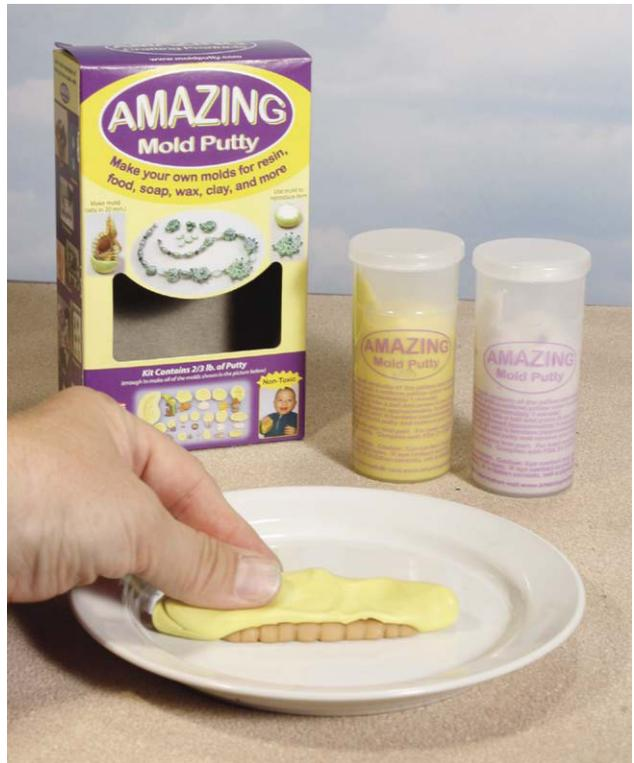
**Figure 6.24** Make a mold of your worm using a material such as Amazing Mold Putty ([www.amazingmoldputty.com](http://www.amazingmoldputty.com)). Blend equal amounts of yellow and white putty together and press over your worm. You will have a cured rubber mold in 25 minutes.
