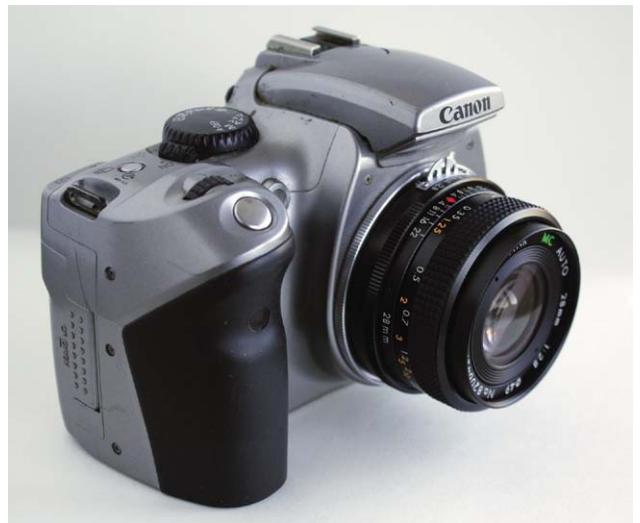
**Figure 10.19** The manual lens attached to the digital camera. You might consider taping the focus down on the lens to prevent it from accidentally being moved.
