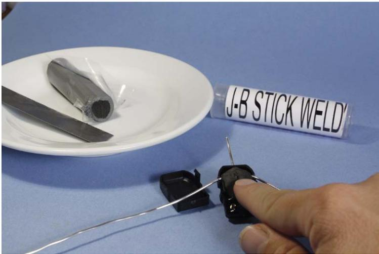
**Figure 5.8** Two-part epoxy putty is a great binder for connecting the aluminum wire to the various parts.
