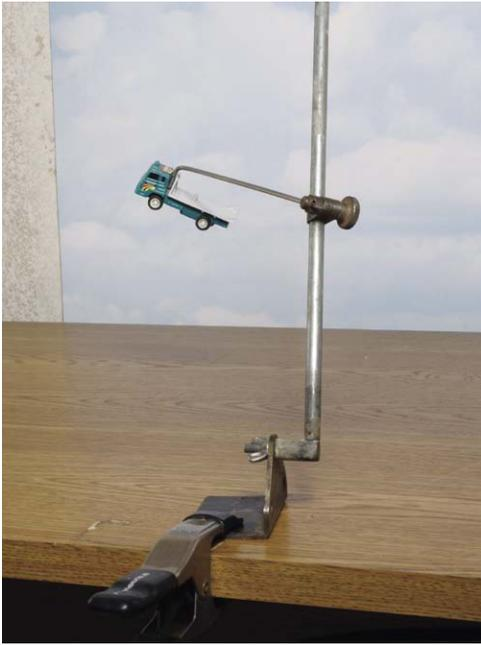
**Figure 3.20** A machinist “surface gauge” can be utilized as a movable support that is easily animated. Note that I chose to support the truck from the top to prevent the support from going over portions of the truck. Erasing supports that go over the model is more time consuming and difficult.
