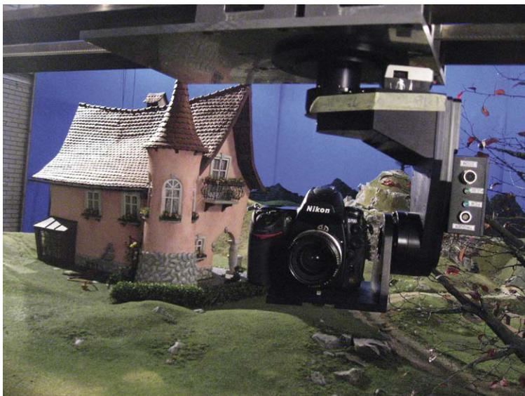
**Figure 11.9** A motion control rig for a Nikon digital camera. Courtesy of Jason Rau of Camera Control, [www.cameracontrol.com](http://www.cameracontrol.com).
