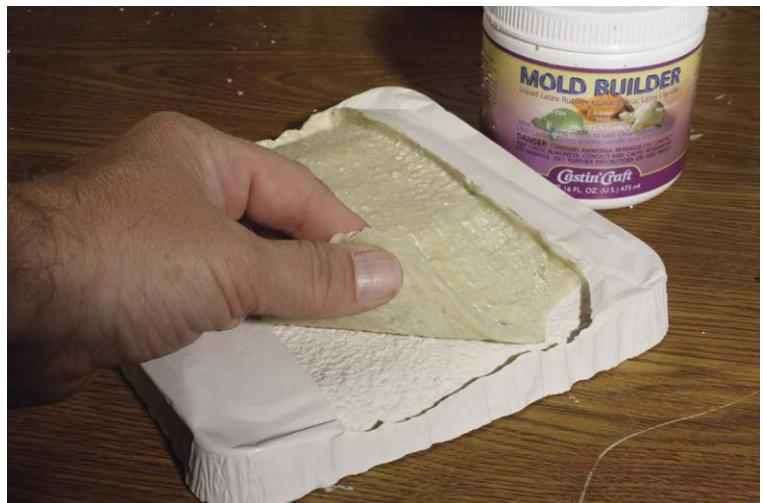
**Figure 7.12** Paint about three or four layers of raw latex into the plaster mold and dry with a heat gun. Dust with talcum powder to prevent the latex from sticking to itself, and remove the textured skin from the mold.
