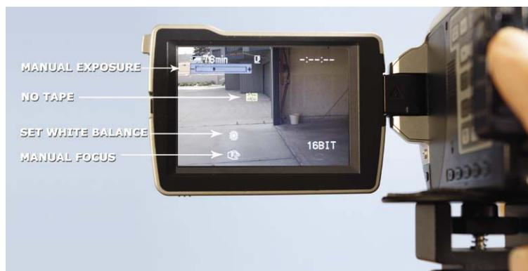
**Figure 2.7** Set the camera white balance for daylight or the outdoor setting. The sun icon should appear. Set your exposure to manual, find a good setting, and leave it alone. This prevents auto exposure fluctuations.
