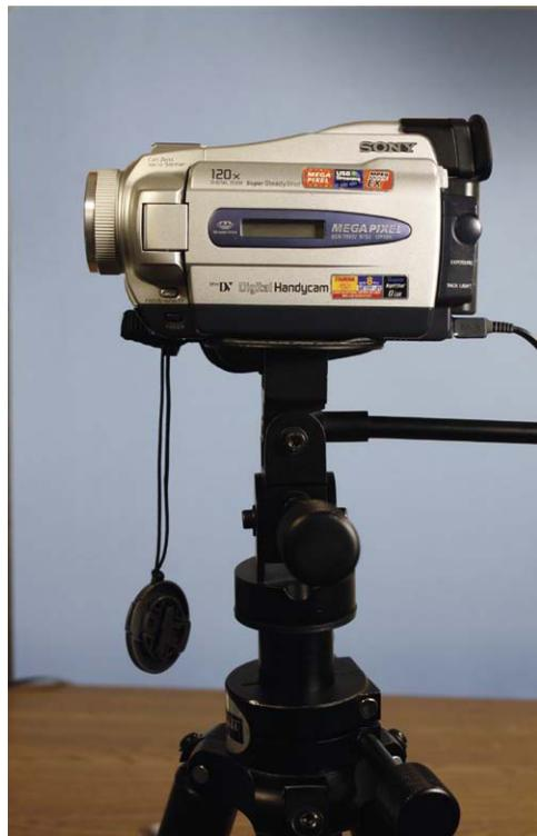
**Figure 2.3** Mount the camera to a sturdy tripod.
