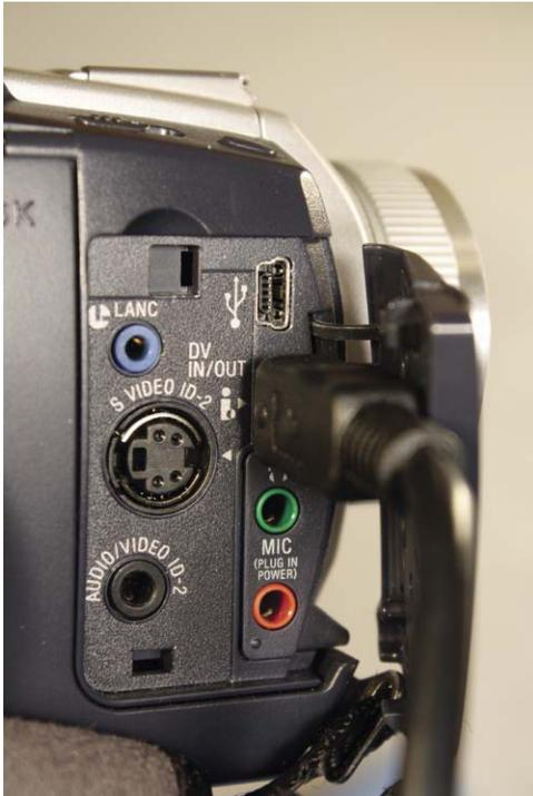
**Figure 2.4** If your camera and computer have an iLink or FireWire cable, you can use that connection. Another solution is to use the video out with the Stop Motion Pro Video Adapter.
