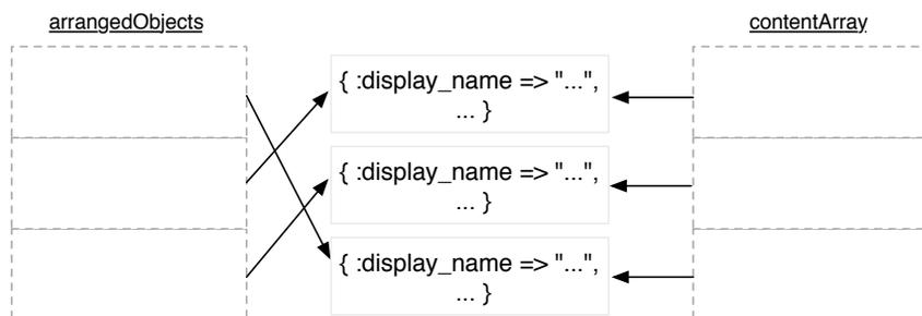
The arrays refer to *the same objects*, just in a different order. Because of `contentArray`'s binding, these objects are identical to the contents of the preference file.
