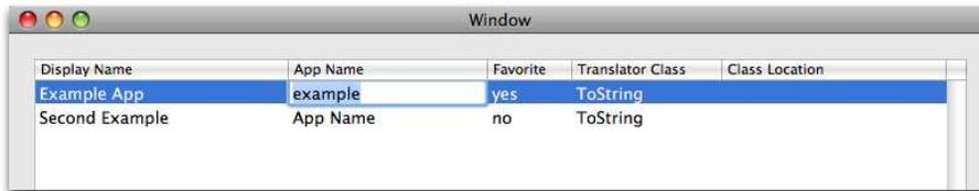
Tabbing goes to a different row, the first one. Why? Here's a clue: continuing to tab moves you from column to column in the first row. Another clue is that the first row is highlighted in the "after" picture, but the second line isn't in "before." Perhaps selecting (as with a single-click) the newly added row would help?
