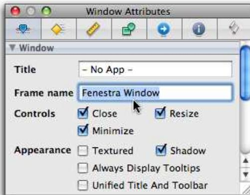
The named window prompts Cocoa to save the window position and size in user preferences. (The frame name is used as the key for that data.)
