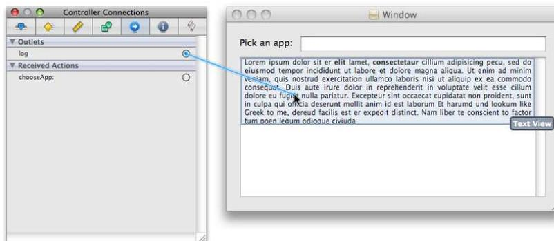
In IB 3.0, the inspector loses track of what it's inspecting when you drop the far end of the connection. Worse, clicking the Controller in the doc window doesn't get it back. What I do is click some other object (like the text view) and then click the Controller again. (Later versions of IB don't have this problem.)
