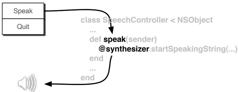
In that code, `@synthesizer` is a particular kind of instance variable: one that points to some Cocoa object used for output. In the jargon, that's an *outlet*.
