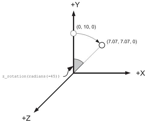
**Figure 9-4.** A rotation about the z axis
