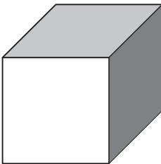
Figure 8-4. A cube rendered with a parallel projection
