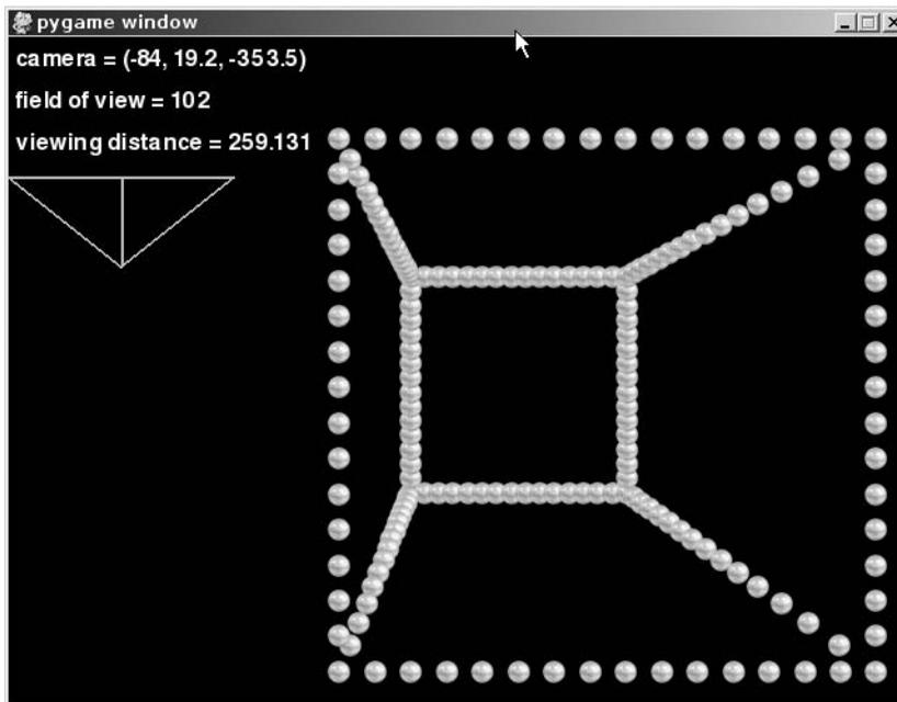
Figure 8-8. A simple 3D engine in Pygame
