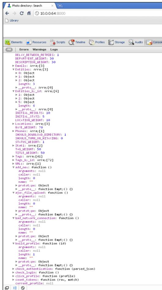
This suggests another explanation, that despite Chrome leading us to believe we have a six-element array, we might have an array of length 6 from JavaScript's perspective, but the keys used to populate it max out at five. It has exactly three physical entries, just like the other. Let's go over to the **Scripts** page and select the **:8000/** entry (the one for JavaScript on the page, although we can see other source files too). That reads as follows:
