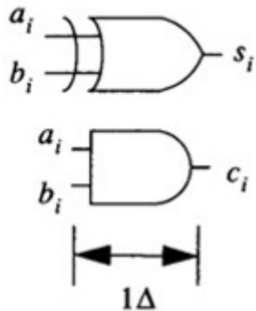
**Figure 4.4** Output Delay Calculation for a Half Adder
