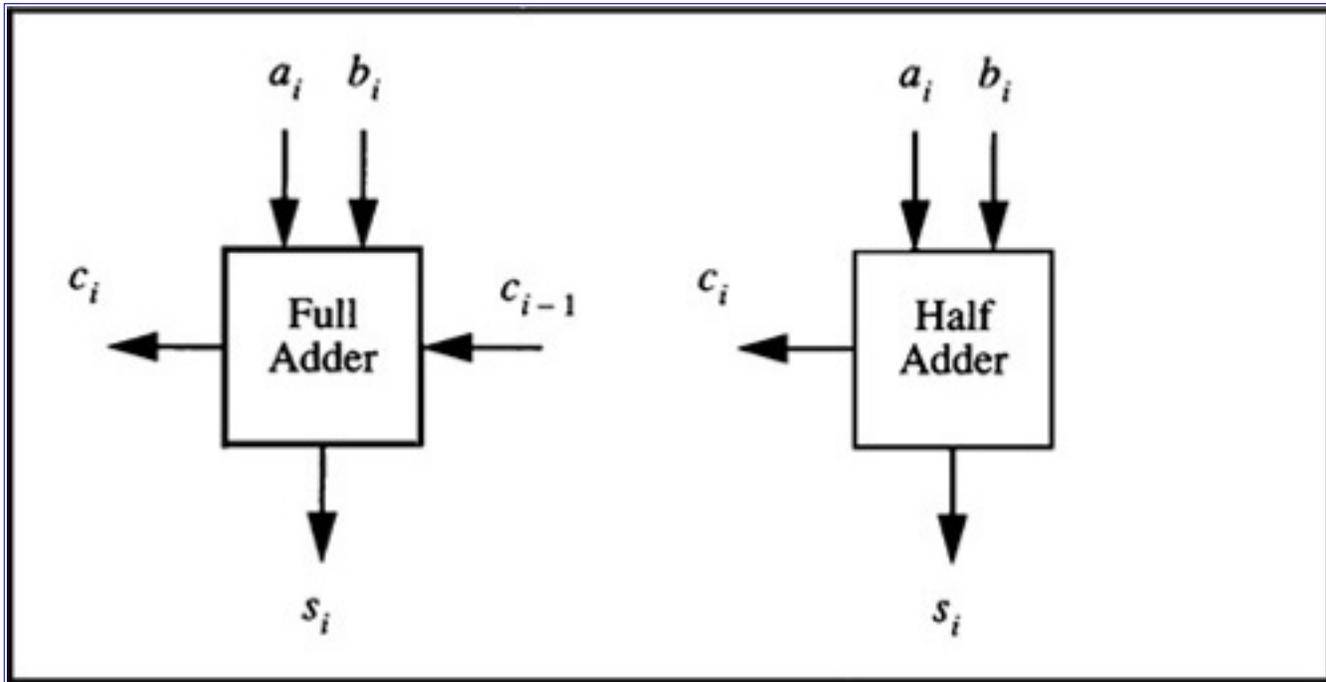
**Figure 4.1** Full and Half Adder Modules
