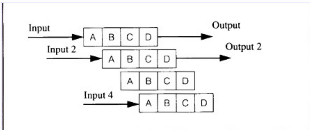
**Figure 2.13** A Four Stage Pipeline
