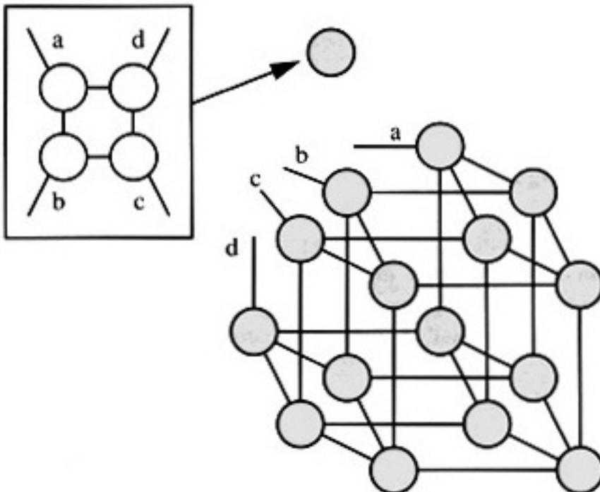
**Figure 2.18** Cube-Connected Cycles
