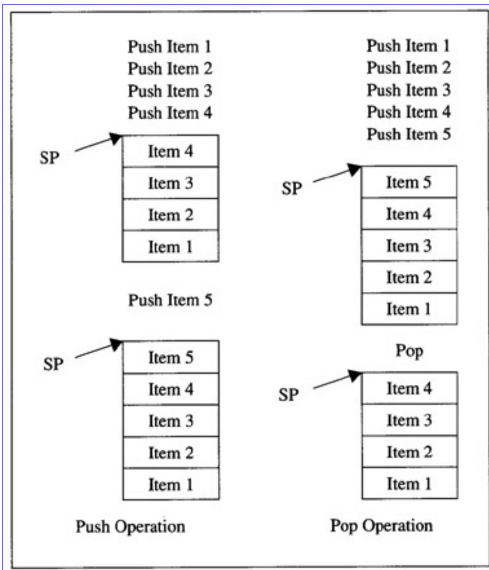
**Figure 3.5** Push and Pop in a LIFO Stack
