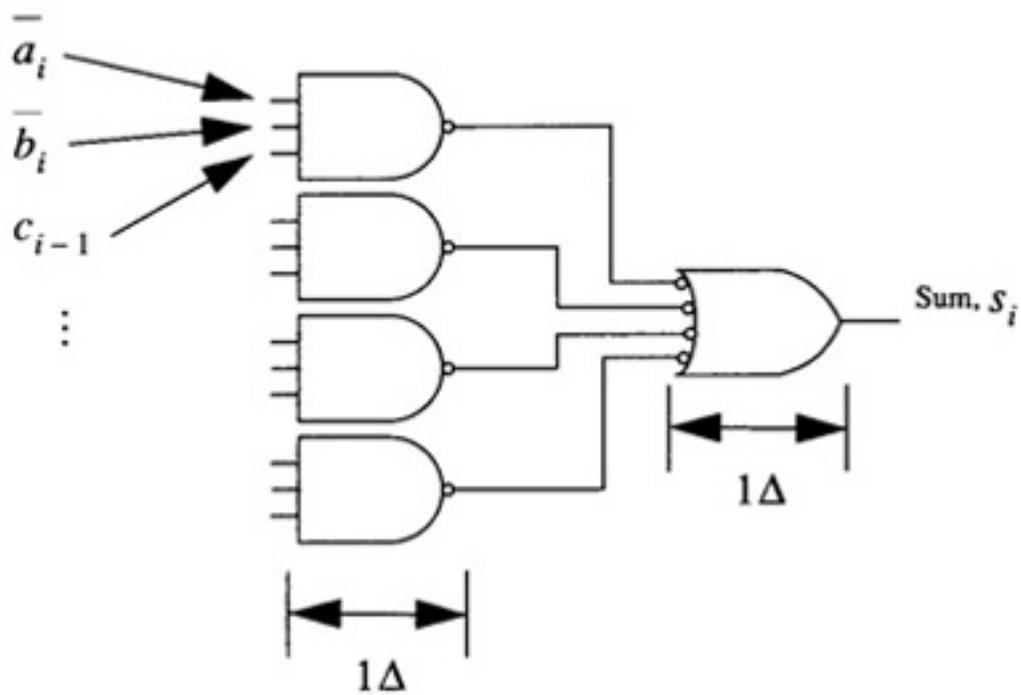
**Figure 4.2** Output Delay Calculation for a Full Adder
