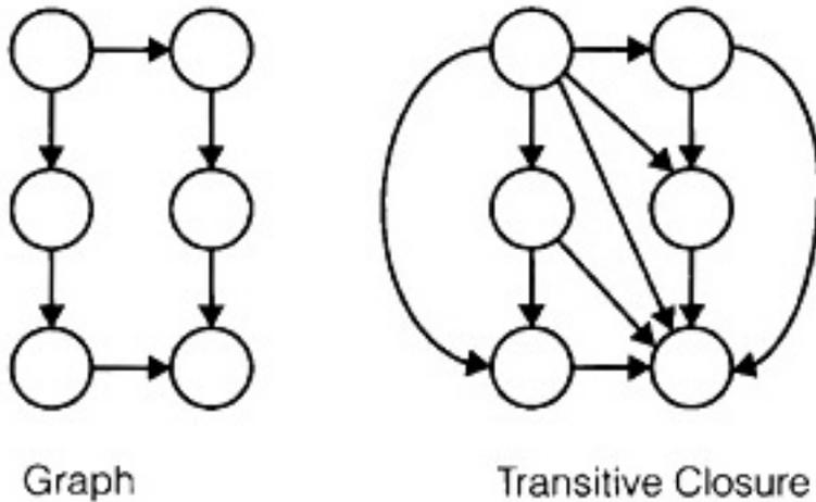
**Figure 2.12** Transitive Closure of a Graph
