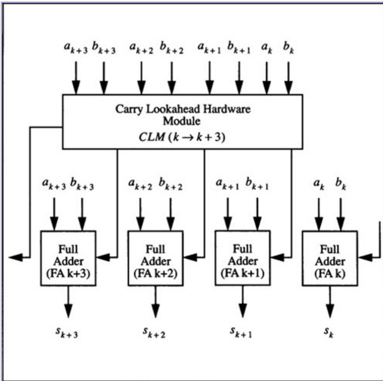
**Figure 4.9** 2's Complement 4-Bit CLA Adder Module
