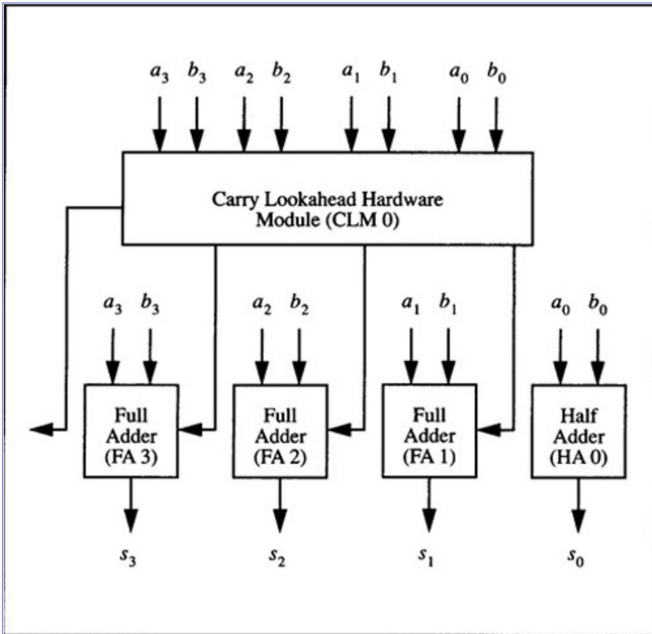
**Figure 4.6** 2's Complement 4-Bit CLA Adder Module
