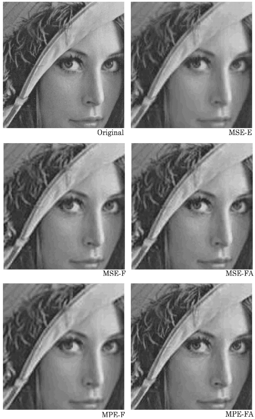
Fig. 6. Compression results on Lena image (0.5 bpp). The figures show the 170 \times 170 central subimage.
