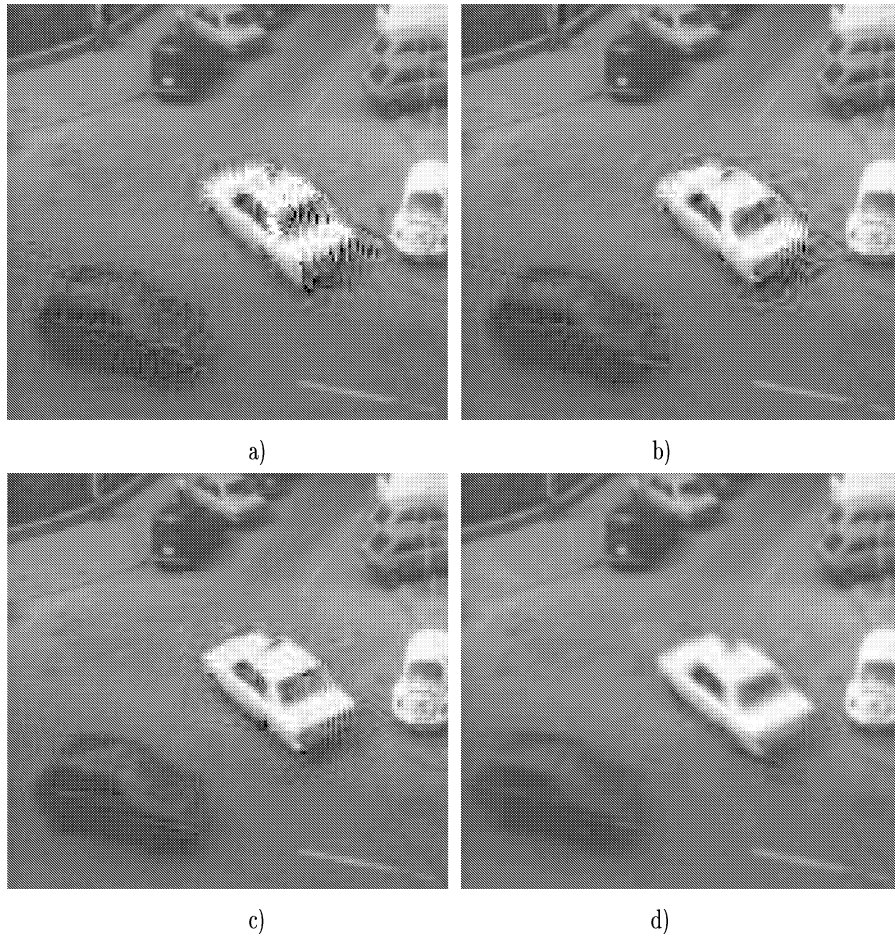
Fig. 10. Zoom of the overall reconstruction results with the TAXI sequence (200 kbits/sec) using previously reported encoding configurations (a-b) and the proposed 2D or 3D alternatives (c-d). a) Fixed size BMA for motion estimation and MPEG-like quantization (linear MPE). b) Unweighted variable-size BMA and MPEG-like quantization (linear MPE). c) Perceptually weighted variable-size BMA and 2D non-linear MPE quantization. d) Perceptually weighted variable-size BMA and 2D non-linear MPE quantization and temporal filtering. The smoothing of the small moving objects in the 3D approach is not as noticeable in the actual (moving) sequences.
