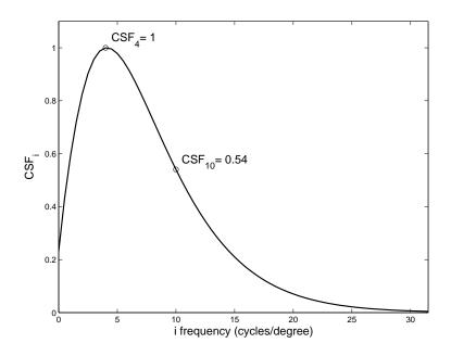
Fig. 1. Contrast Sensitivity Function (CSF) of Nygan et al. [28]. The slopes of two particular sensors respectively tuned to low-frequency stimuli (CSF<sub>4</sub> = 1) and high-frequency stimuli (CSF<sub>10</sub> = 0.54) have been highlighted.
