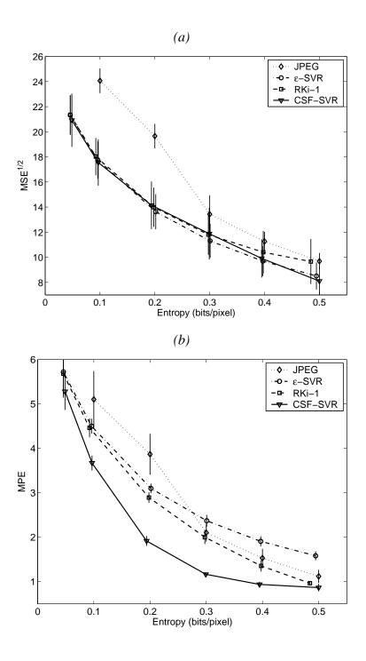
Fig. 4. Rate distortion curves of JPEG and the three SVM-based image coding methods. (a) Distortion measured with the standard  $MSE^{1/2}$ . (b) Distortion measured using the perceptually meaningful MPE. These results are the average over the five standard images, and the error bars stand for the standard deviation of the corresponding distortion at each point.
