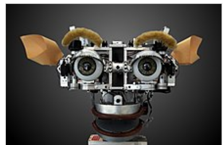
Kismet , a robot head which was made in the 1990s; it is a machine that can recognize and simulate emotions. [64]
