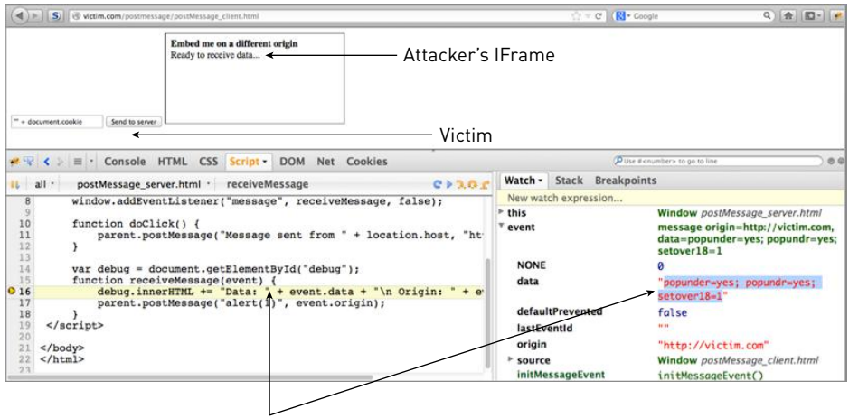
Breakpoint on the framed attacker's code. Note the 'data' variable content.
