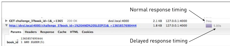
Figure 9-11: Time delay of a successful SQLi attack
