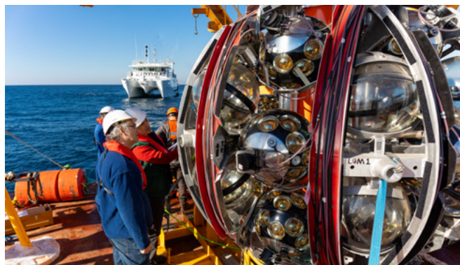
Launching of the ORCA lines optical modules for the KM3Net neutrino detector, a second-generation neutrino telescope. © Patrick Dumas - CNRS Photothèque
