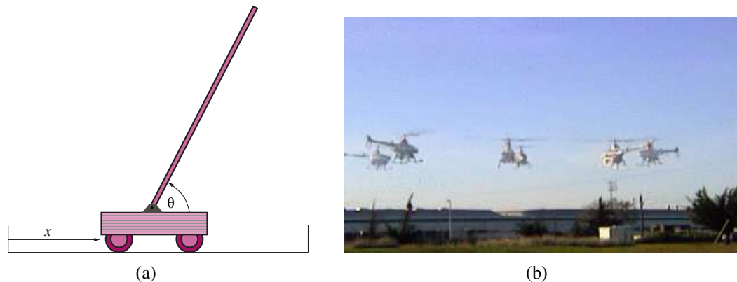
Figure 23.9 (a) Setup for the problem of balancing a long pole on top of a moving cart. The cart can be jerked left or right by a controller that observes the cart’s position x and velocity \dot{x} , as well as the pole’s angle \theta and rate of change of angle \dot{\theta} . (b) Six superimposed time-lapse images of a single autonomous helicopter performing a very difficult “nose-in circle” maneuver. The helicopter is under the control of a policy developed by the PEGASUS policy-search algorithm (Ng et al. , 2003). A simulator model was developed by observing the effects of various control manipulations on the real helicopter; then the algorithm was run on the simulator model overnight. A variety of controllers were developed for different maneuvers. In all cases, performance far exceeded that of an expert human pilot using remote control. (Image courtesy of Andrew Ng.)
