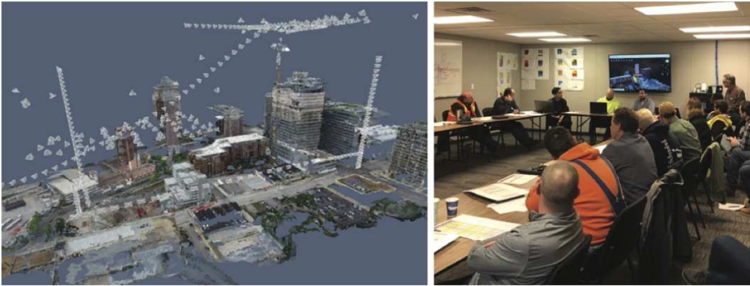
Figure 27.21 3D models of construction sites are produced from images by structure-from-motion and multiview stereo algorithms. They help construction companies to coordinate work on large buildings by comparing a 3D model of the actual construction to date with the building plans. Left: A visualization of a geometric model captured by drones. The reconstructed 3D points are rendered in color, so the result looks like progress to date (note the partially completed building with crane). The small pyramids show the pose of a drone when it captured an image, to allow visualization of the flight path. Right: These systems are actually used by construction teams; this team views the model of the as-built site, and compares it with building plans as part of the coordination meeting. Figure courtesy of Derek Hoiem, Mani Golparvar-Fard and Reconstruct, produced by a commercial system described in a blog post at medium.com/reconstruct-inc .
