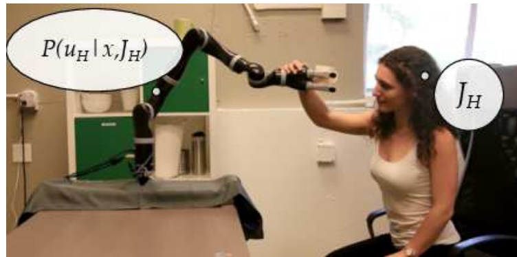
Figure 26.30 A human teacher pushes the robot down to teach it to stay closer to the table. The robot appropriately updates its understanding of the desired cost function and starts optimizing it. Courtesy of Anca Dragan. See Bajcsy et al. (2017).
